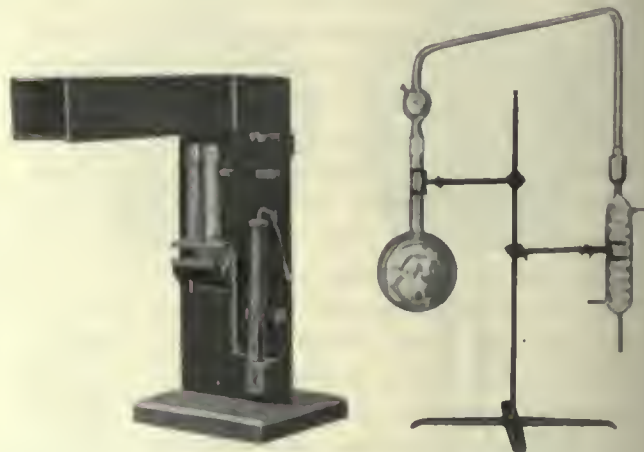
FIG. 69. TINTOMETER AND APPARATUS USED FOR DISTILLING AMMONIA
